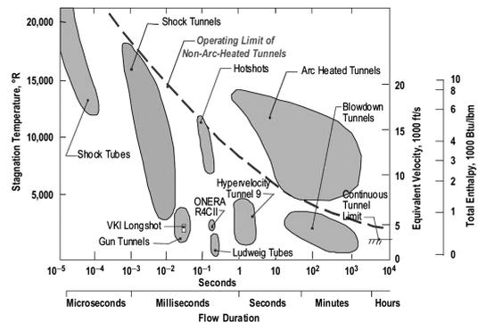
Fig. 11 Unique role of arc heater facility
