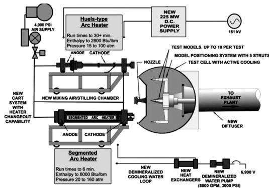
Fig. 13 Proposed new facility with huels and segmented heaters
