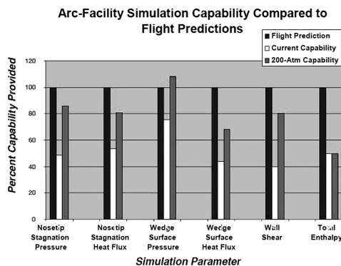
Fig. 15 Comparison between flight conditions and  $H_3$  arc heater test conditions
