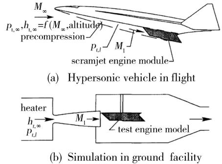
Fig. 5 Ground test simulation of flight for scramjet engine testing
