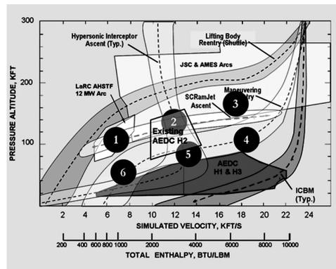
Fig. 12 USA National mission operating points and existing ground simulation capability
