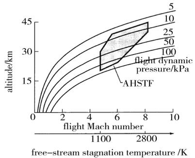
Fig. 6 Simulation capability of AHSTF
