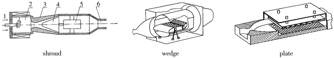
Fig. 10 Sketch of test techniques in TSNIIMASH arc heater facility
