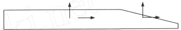
图 2 变厚度层板成型过程中树脂流动示意图 Fig 2 Sketch map of resin flow during processing in variable thickness laminates
