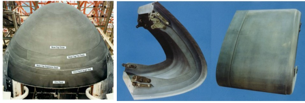
图 11 航天飞机抗氧化 C/C 材料头锥和翼前缘 Fig. 11 Anti-oxidation C/C nose cap and leading edge of the space shuttle
