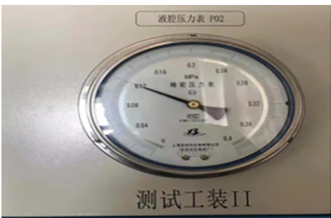
图7 测试工装 II 液腔压力表显示值 Fig. 7 The display value of the pressure gauge for the test fixture II in the liquid chamber
