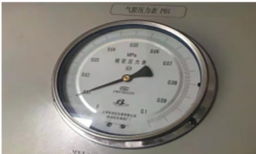
图5 测试工装 I 气腔压力表显示值 Fig. 5 The display value of the pressure gauge for the test fixture I in the air chamber
