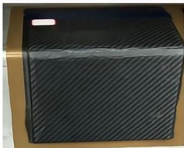
图6 固化完成后的L形构件 Fig. 6 The L-shaped model after curing
