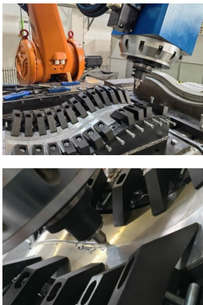
图13 机器人搅拌摩擦焊系统进行S形空间曲线焊接过程 Fig. 13 The S-shaped space curve welding process of robot friction stir welding system
