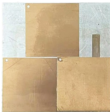
图9 Parylene-C 薄膜经 1 \times 10^{14} \text{ e/cm}^2 电子辐照后外观 Fig. 9 Appearance of Parylene-C films after 1 \times 10^{14} \text{ e/cm}^2 electron irradiation
