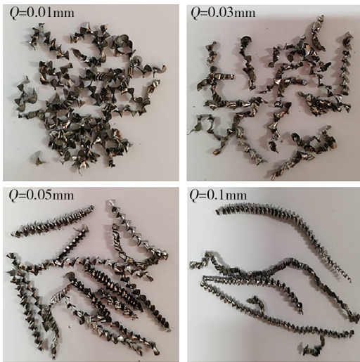
图9 CFRP/TC4叠层结构啄式钻削工艺下的钛合金切屑形态 Fig. 9 Titanium alloy chip morphology under CFRP/TC4 stacks structure pecking drilling process
