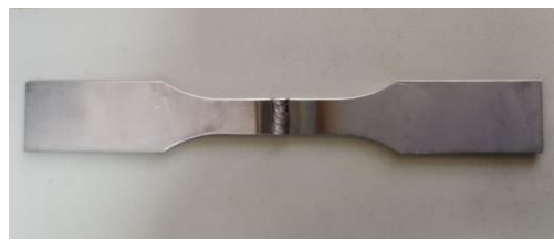
(a) Welded joint specimen
