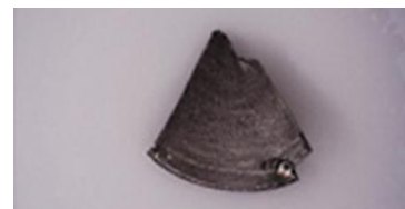
(c) 低频振动钻削的切屑形态
