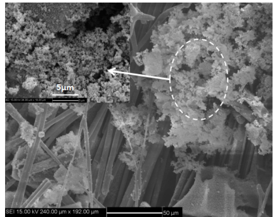
图6 HRC-3烧蚀后碳化层微观形貌SEM照片 Fig. 6 SEM image of charred layer for HRC-3 sample after ablation
