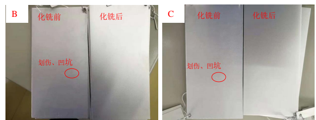
图2 6A02-B、6A02-C化铣前后表面质量 Fig. 2 The surface quality of 6A02-B, 6A02-C before and after chemical milling
