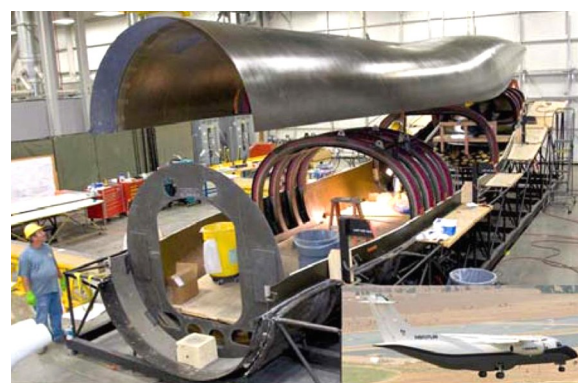
图 3 MTM45-1 材料用于 ACCA 大型整体化机身结构 Fig. 3 Application of MTM45-1 material in ACCA aircraft fuselage structure
