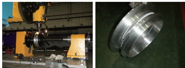
图 17 异种铝合金部件对接环缝的可回抽搅拌摩擦焊接 Fig. 17 Reversible friction stir welding of butt joint of dissimilar aluminum alloy components
