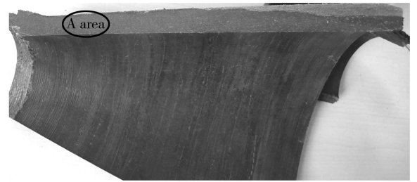
(a) Cross section of angled tape wrapping exit cone for \Phi 315 mm motor
