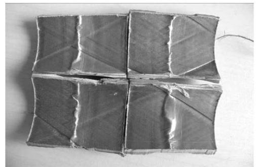
(c) F-3A 纤维轴压试样解剖形貌
