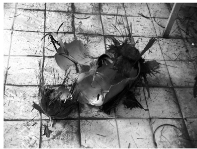
Fig.2 Photographs of the composite vessel after blast test
