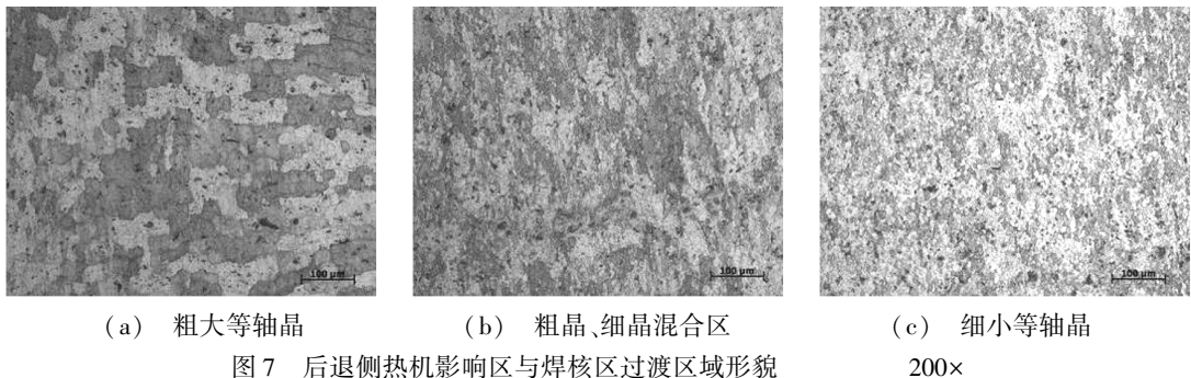
Fig. 7 Morphologies between NZ and retreating TMAZ
