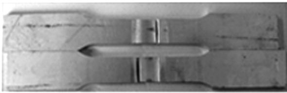
图8 匙孔修补位置与二次焊接区拉伸断裂形貌 Fig.8 Fracture specimen after tensile test at different position of repaired FSW joint
