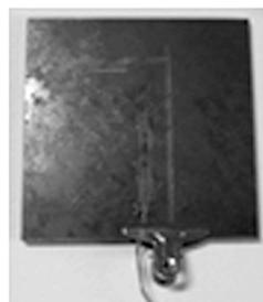
(c) 6 mm glass fiber reinforced phenolics before test
