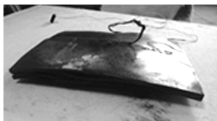
(e) 6 mm glass fiber reinforced phenolics after test
