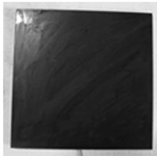
(b) 6 mm glass fiber reinforced phenolics before test
