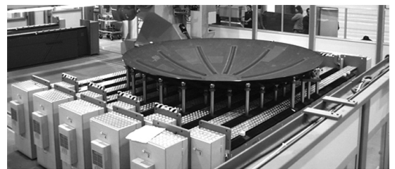
图 8 A340 机身气密舱球面框 [6] Fig. 8 Pressure bulkhead of A340-600 [6]
