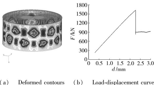
Fig.4 Analysis results of orthogrid cylindrical shell
