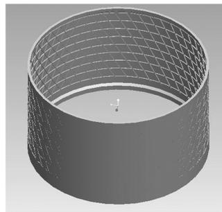
Fig.5 3D model of isogrid C/E CTWS
