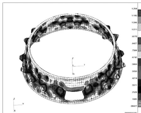
(a) Structure could buckle in complete cycle
