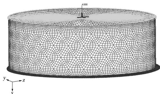
Fig. 1 Finite element model of isogrid C/E CTWS cylindrical shell
