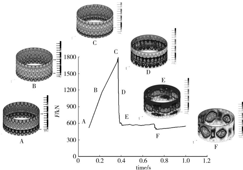
Fig.2 Typical load-displacement curve of isogrid C/E CTWS cylindrical shell under quasi-static axial compression
