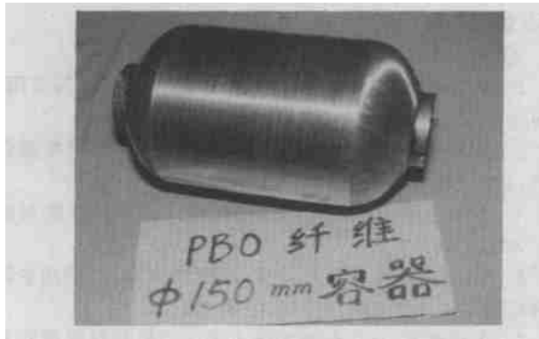
图 4 干法缠绕成型 150 mm 压力容器 Fig. 4 Photograph of pre-preg filament wound 150 mm pressure vessel
