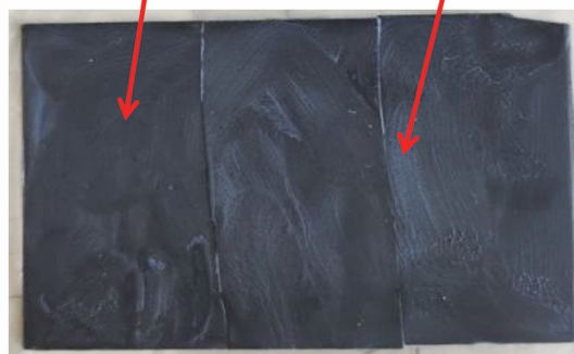
图3 全氟醚橡胶试片涂抹润滑脂后的微观形貌 Fig. 3 The microscopic morphology of perfluoroether rubber specimens after coated with grease
