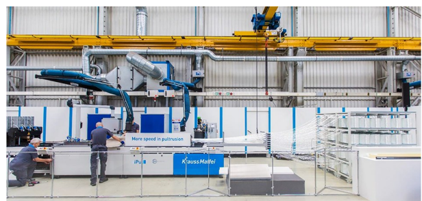
图9 德国的Krauss Maffei等公司研发的iPul连续拉挤生产线 [48] Fig. 9 The iPul continuous extrusion production line developed by German companies such as Krauss Maffei [48]
