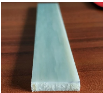
图5 拉挤成型的玻璃纤维增强聚合热塑性PA-6构件 [42] Fig. 5 Glass fiber reinforced thermoplastic PA-6 components fabricated by pultrusion process [42]
