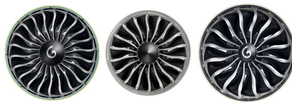
图6 GE公司三款发动机中风扇叶片的数量对比 Fig. 6 Comparison of the amount of fan blades of GE's three latest engines
