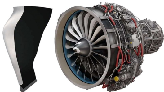
图7 LEAP发动机及其复合材料风扇叶片 Fig. 7 LEAP engine and its composite fan blade
