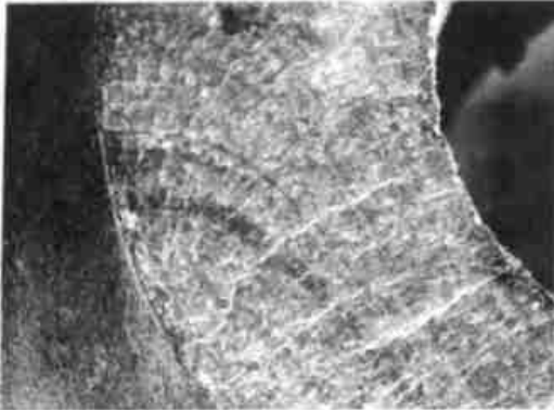
图1 箭头所示主疲劳源区附近的疲劳弧线 30 × Fig. 1 Camber lines near the main initiation zone
