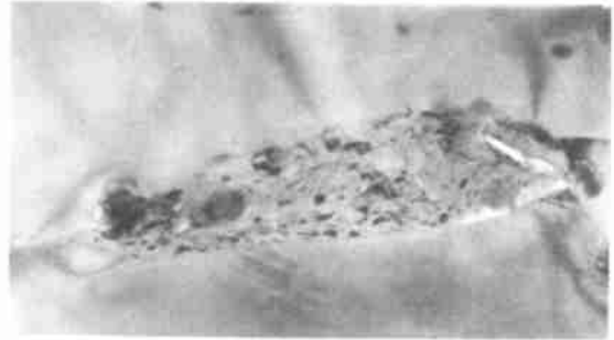
图 4 B_4C_p /Al 复合材料 TEM 照片 35 000 × Fig. 4 TEM micrograph of the B_4C_p /Al composites
