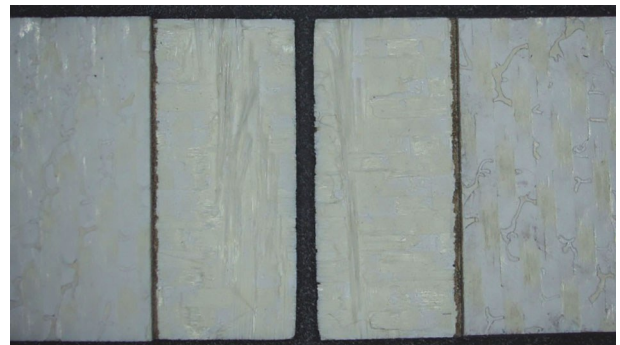
图 13 \text{Al}_2\text{O}_3/\text{Al}_2\text{O}_3 复合材料层剪试样断口形貌 Fig. 13 Fracture surface of \text{Al}_2\text{O}_3/\text{Al}_2\text{O}_3 composite specimens after shear test
