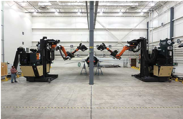
图14 激光涂层去除系统对F-16战斗机进行激光除漆 Fig. 14 Laser paint removal of F-16 fighter by laser coating removal system
