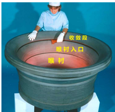
图1 P230喷管A C/C喉衬实物 Fig. 1 C/C throat of P230 nozzle-A
