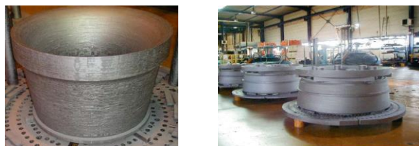
图2 P230喷管B C/C喉衬毛坯图 Fig. 2 C/C throat of P230 nozzle-B
