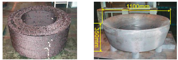
图 5 M-V 一级喉衬预制体及 C/C 喉衬实物 Fig. 5 M-V first stage throat preform and C/C throat
