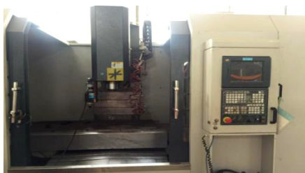
图4 数控超声波喷丸成形设备 Fig.4 Numerical control ultrasonic peening forming equipment
