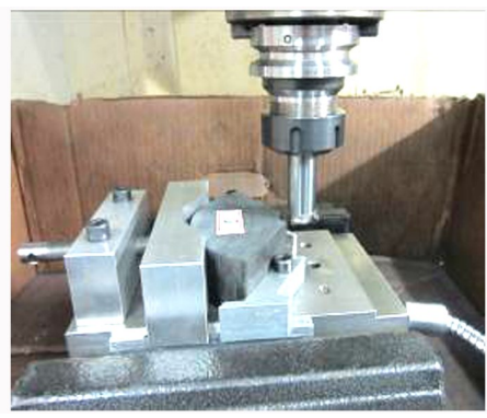
Fig.3 Experimental setup and clamp of workpieces
