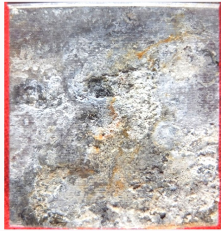
(b) cracked surface of stainless steel
