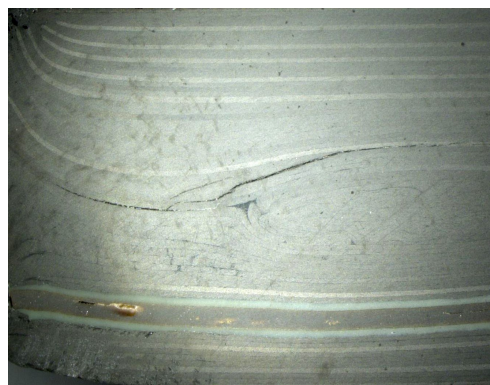
图 8 分层缺陷产品解剖图 Fig.8 Cross-section of product with delamination defects
