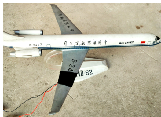
图9 飞机机翼的除冰 Fig.9 Deicing of aircraft wing
