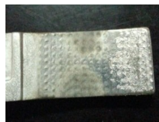
图9 曲面电极加工工件表面 Fig. 9 Surface of workpiece machined by curved electrode
